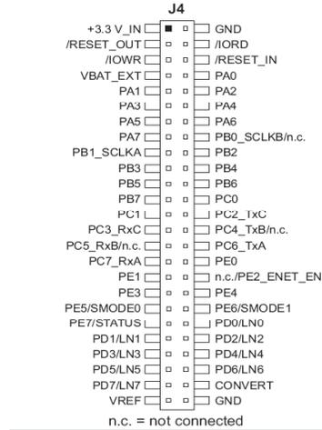
*Note: These pinouts are as seen on the Bottom Side of the module.*
