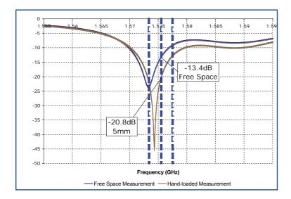
Immunity from bio-loading effects can be demonstrated effectively through the S11 plot. While some change in match is observed as a phantom hand is moved closer to the radiating section of the antenna, minimal de-tuning occurs.
