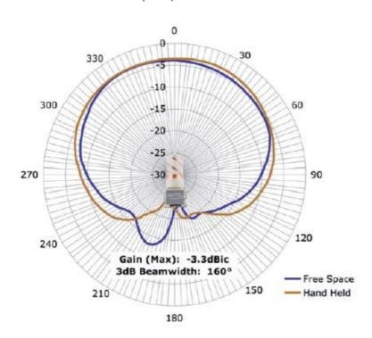
The strength of the PowerHelix antenna technology is its immunity to de-tuning in the presence of dielectric loading, like human tissues. The GeoHelix-SMP antenna retains efficiency and polarization near the human body. Conventional antennas lose 5-10dB of gain in similar circumstances.
