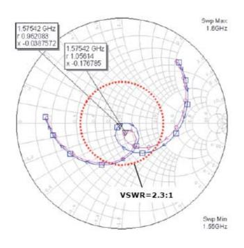
The GeoHelix-SMP antenna is optimized for 50  $\Omega$  impedance to simplify the matching process. The Smith chart showing a typical impedance plot of the GeoHelix-SMP has been normalized to 1. The resonant frequency of the antenna is shown at the markers, and the bandwidth of the antenna is shown by the dimensions of the loops. The red circle shows the VSWR<=2.3:1 impedance mask.
