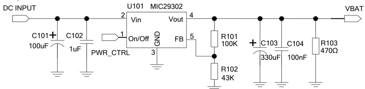
Figure 6: Reference circuit of the power supply
