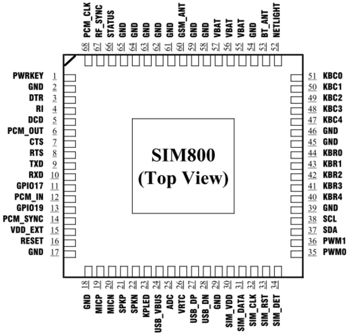
Figure 2: SIM800 pin out diagram (Top view)
