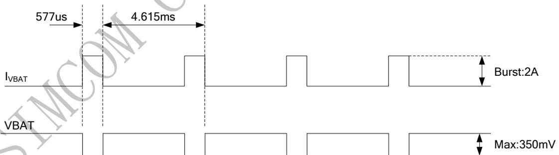
Figure 8: VBAT voltage drop during transmit burst
