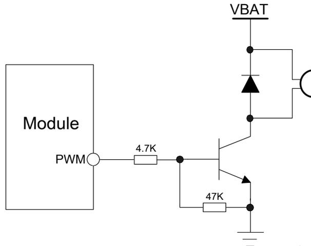
Figure 42: Reference circuit of PWM drive buzzer
