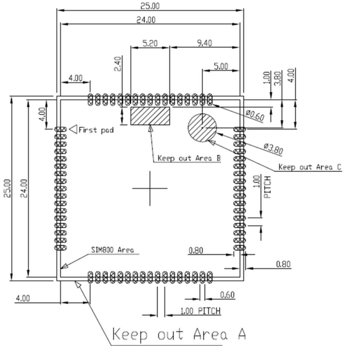
Figure 4: Recommended PCB footprint outline (Unit: mm)
