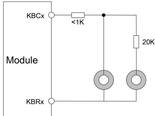
**Figure 39: Enhance the ESD performance of keypad circuit**
