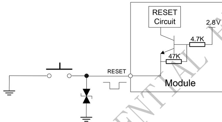
Figure 14: Reset circuit
