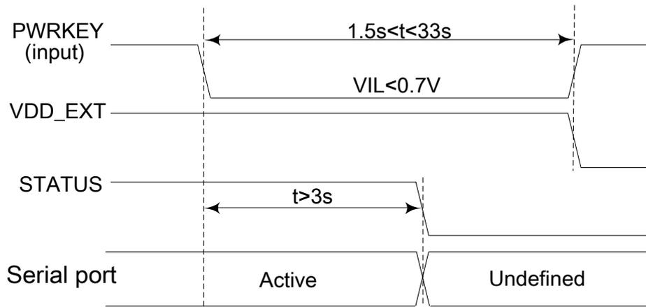
**Figure 13: Timing of Power off SIM800 by PWRKEY**
