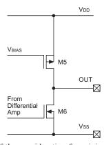
Because of the consideration for minimized power consumption, the output short circuit current is limited to about -1.2mA for source drive and 4mA for sink drive. This is believed to be enough for most low power systems, however it is recommended to use the load resistor of >1M $\Omega$  for normal applications. In case of heavy load driving, an external buffer stage using bipolar transistors is recommended.
