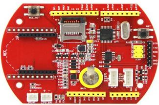
Seeeduino Stalker v3 is an Arduino compatible main board which has various functions. It's an X-Bee carrier board while using with X-Bee modules, such as GPS Bee, Bluetooth Bee and Wifi Bee, etc. It's a charger for Lipo while plugging a solar panel onto the board. Also, you can get time from the inside RTC chip, and all data can be easily stored through the SD card. In a word, Seeeduino Stalker v3 has an independent ecological system and it's good for applications in outdoor environment.
