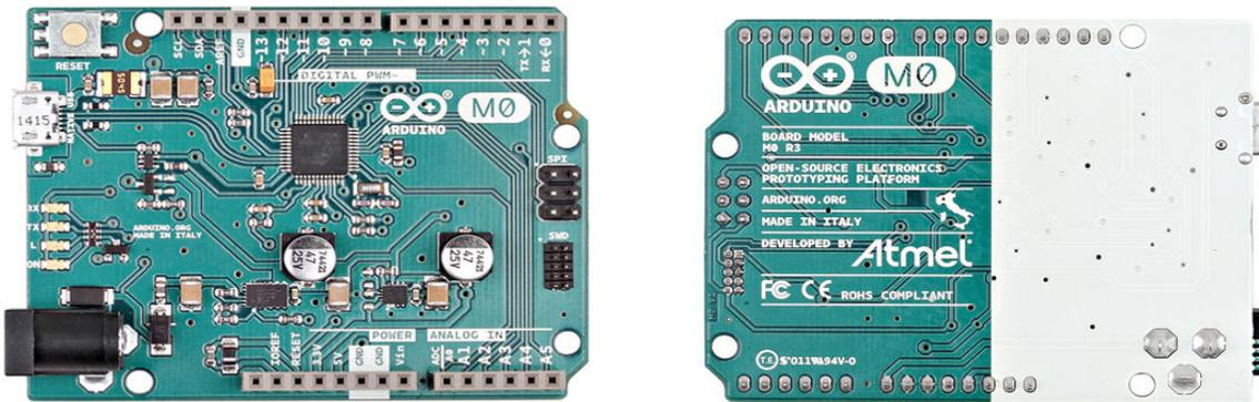
The Arduino M0 is ideal for projects demanding high computing power. It features a Cortex M0+ running at 48MHz clock speed. All digital pins have PWM capability. It also has a real digital to analog conversion making it ideal for sound applications
