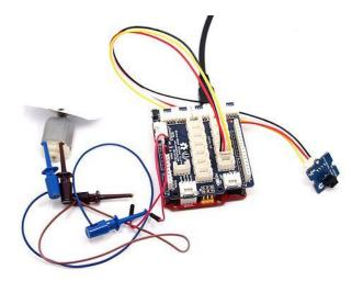
**Note:**Add a white plate with a black line marked onto the motor so that the sensor can get one signal when the plate rotates a round.
