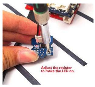
After that, keep the distance and move the sensor horizontally above the black line. if the indicator
