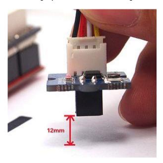
Then adjust the potentiometer with a crosshead screwdriver until the indicator LED turns on.
