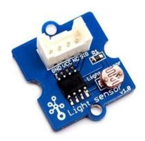
The light sensor, also known as the light dependent resistor (LDR). Typically, the resistance of the
