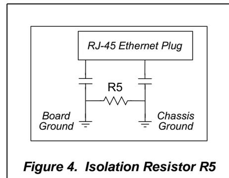
**Figure 4. Isolation Resistor R5**
