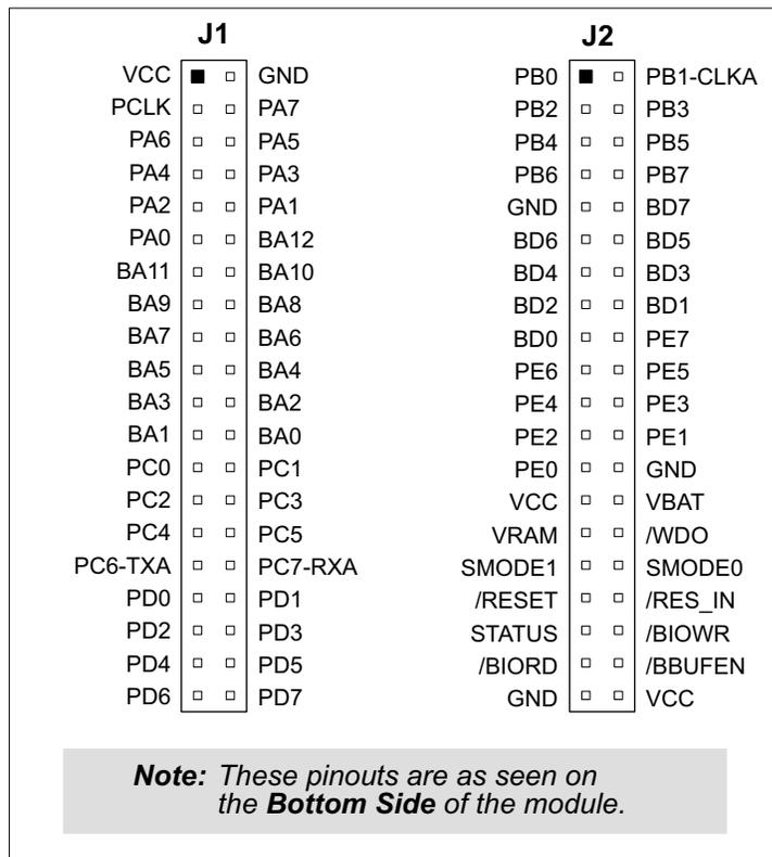
**Figure 2. RCM2100 I/O Pinouts**
