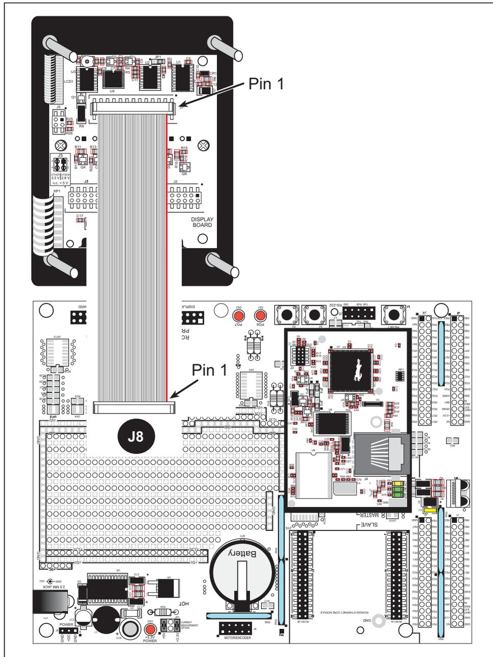
**Figure C-10. Connecting LCD/Keypad Module to RCM30/31/32XX Prototyping Board**
