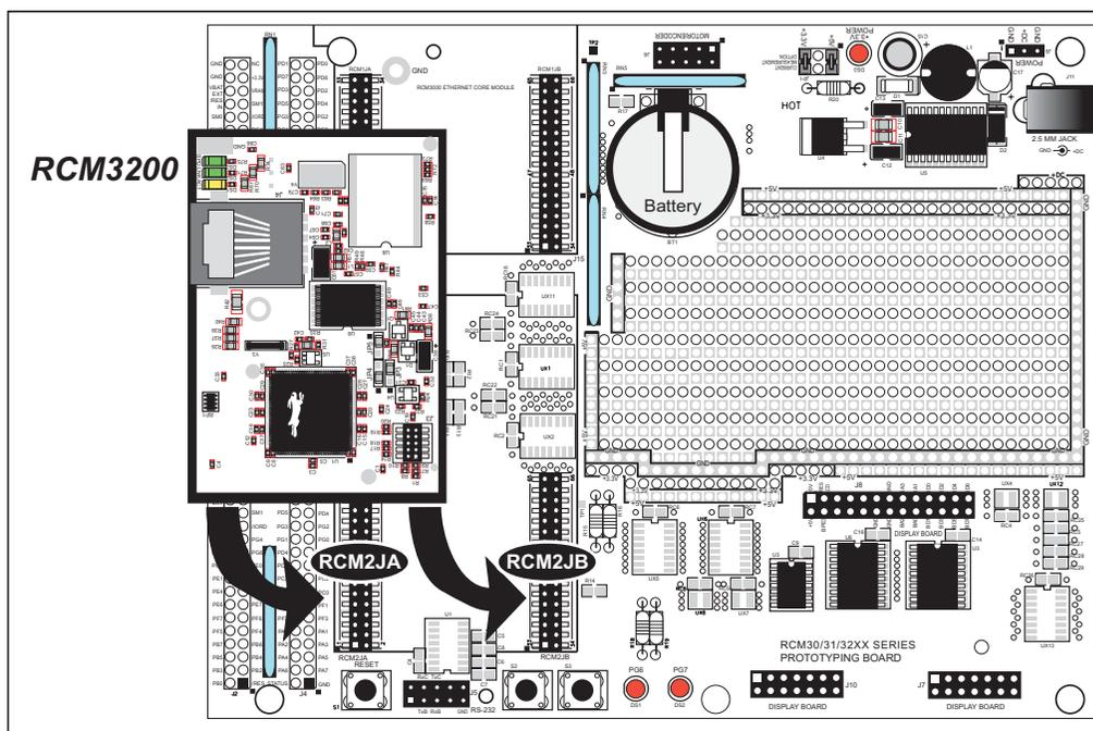
**Figure 1. Installing the RCM3200 Module on the Prototyping Board**
