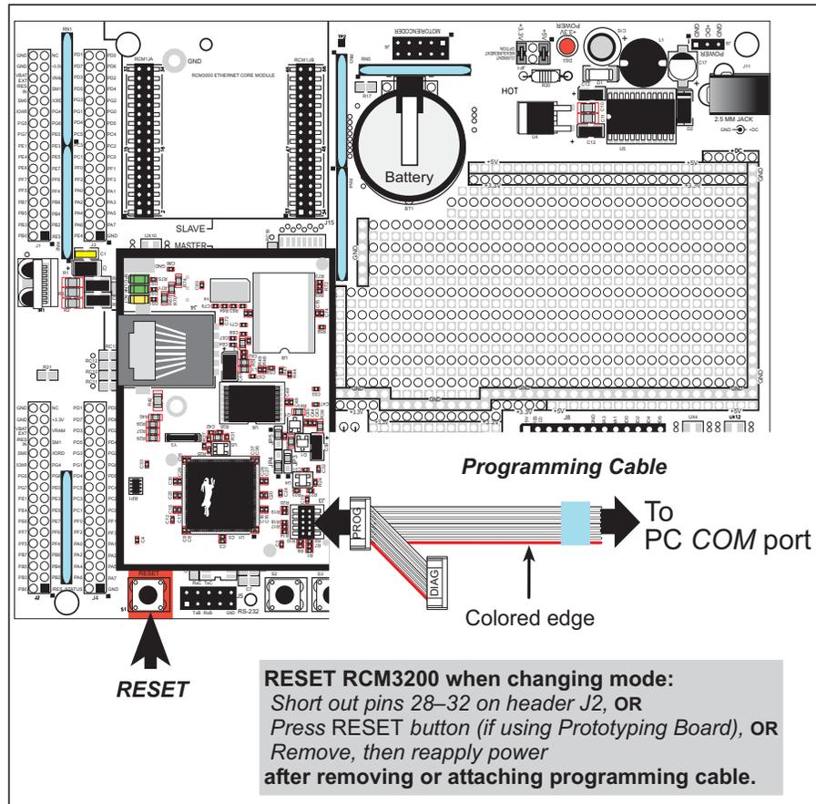
Figure 9. Switching Between Program Mode and Run Mode
