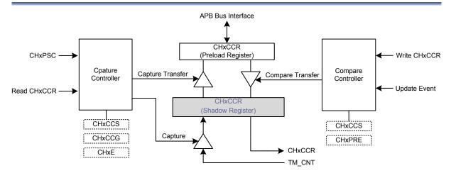
Figure 41. Capture/Compare Block Diagram
