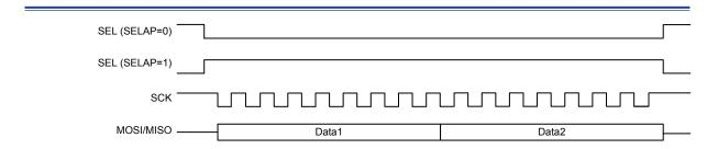
Figure 104. SPI Continuous Transfer Timing Diagram - CPOL = 1, CPHA = 1
