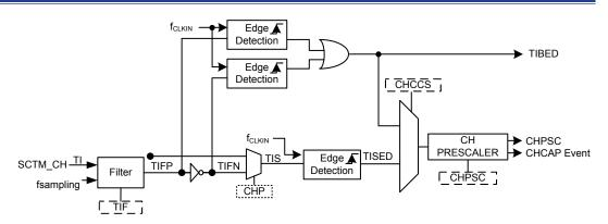
Figure 73. Channel Input Stages
