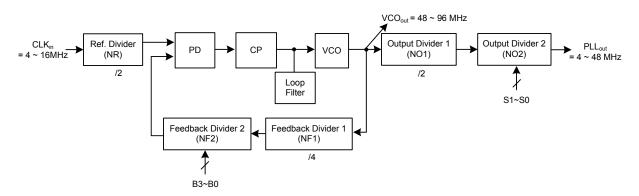
Figure 15. PLL Block Diagram
