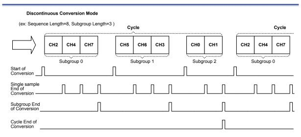
Figure 28. Discontinuous Conversion Mode
