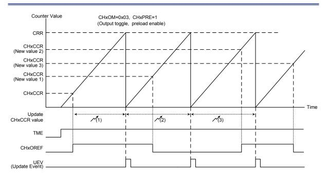
Figure 51. Toggle Mode Channel Output Reference Signal – CHxPRE = 1
