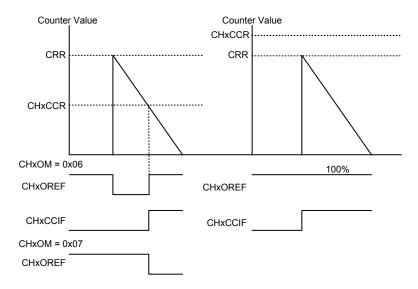
Figure 53. PWM Mode Channel Output Reference Signal and Counter in Down-counting Mode
