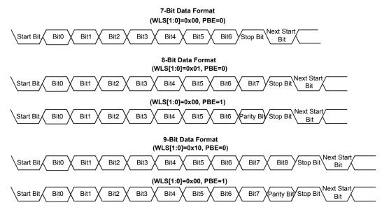
Figure 118. UART Serial Data Format
