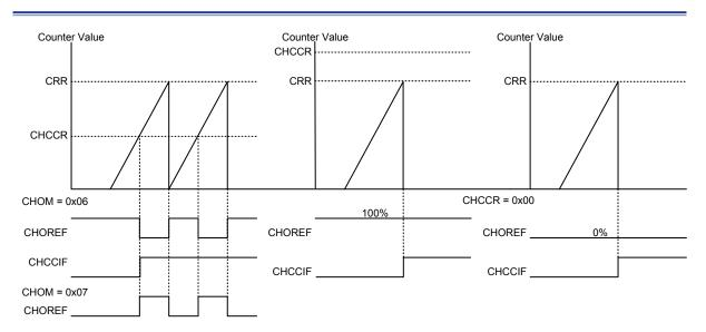
Figure 78. PWM Mode Channel Output Reference Signal
