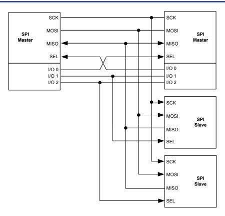
Figure 105. SPI Multi-Master Slave Environment
