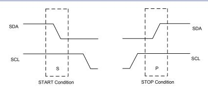
Figure 83. START and STOP Condition
