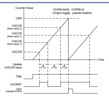
Figure 76. Toggle Mode Channel Output Reference Signal – CHPRE = 0
