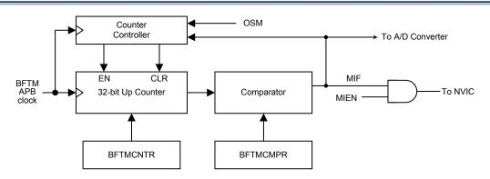
Figure 59. BFTM Block Diagram
