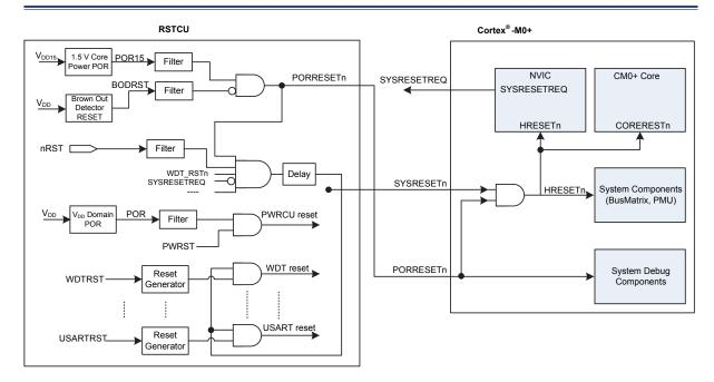
Figure 16. RSTCU Block Diagram
