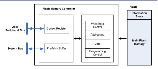
Figure 5. Flash Memory Controller Block Diagram
