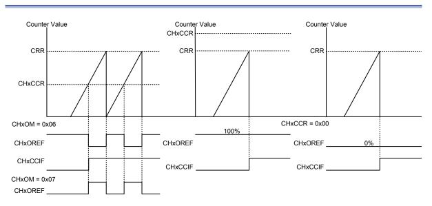
Figure 52. PWM Mode Channel Output Reference Signal and Counter in Up-counting Mode
