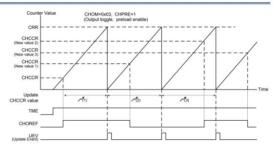
Figure 77. Toggle Mode Channel Output Reference Signal – CHPRE = 1
