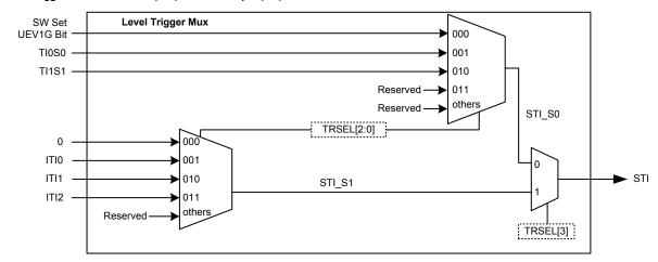
Figure 34. Trigger Controller Block
