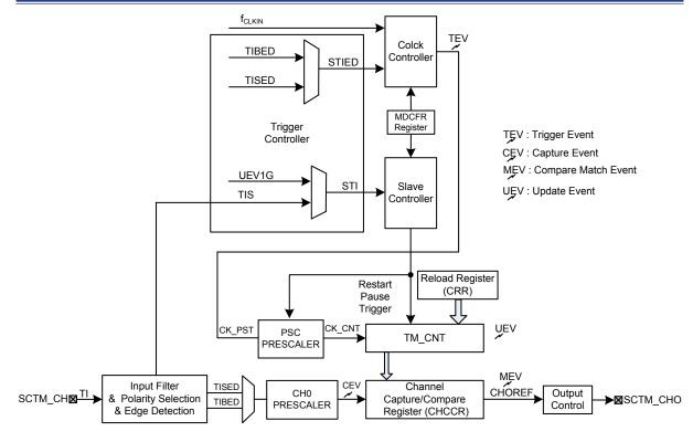
Figure 63. SCTM Block Diagram
