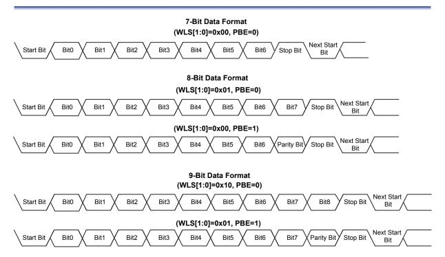
Figure 107. USART Serial Data Format
