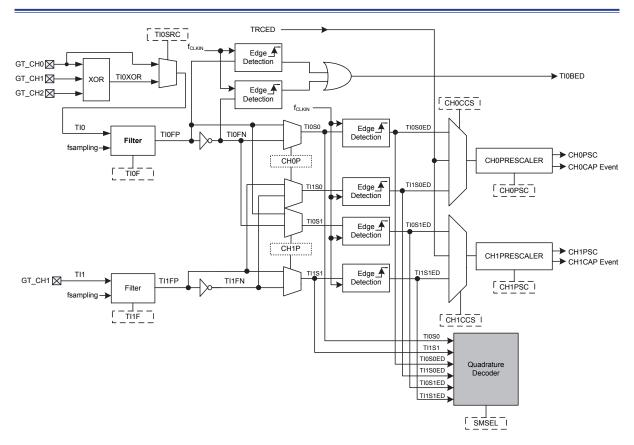
Figure 47. Input Stage and Quadrature Decoder Block Diagram
