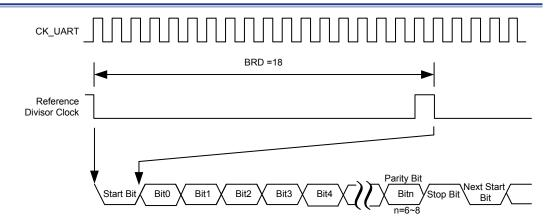
Figure 119. UART Clock CK\_UART and Data Frame Timing
