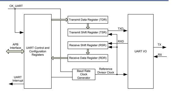
Figure 117. UART Block Diagram
