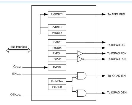
Figure 18. GPIO Block Diagram
