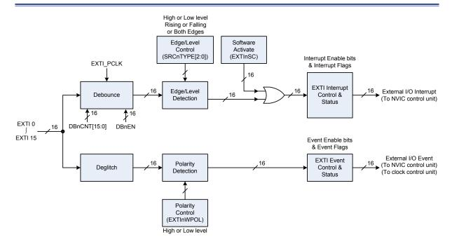
Figure 22. EXTI Block Diagram
