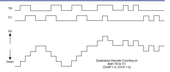
Figure 48. Both TI0 and TI1 Quadrature Decoder Counting
