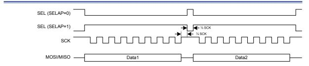
Figure 102. SPI Continuous Transfer Timing Diagram - CPOL = 1, CPHA = 0
