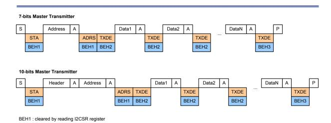
Figure 91. Master Transmitter Timing Diagram
