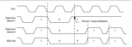
Figure 90. Two Master Arbitration Procedure
