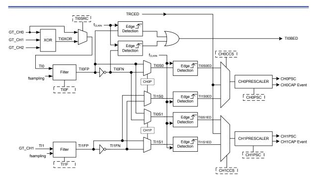
Figure 44. Channel 0 and Channel 1 Input Stages
