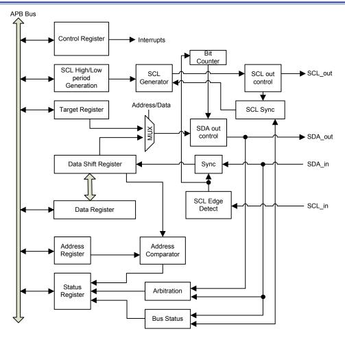
Figure 82. I<sup>2</sup>C Module Block Diagram
