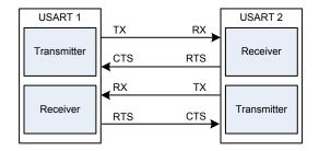
Figure 109. Hardware Flow Control between 2 USARTs
