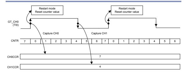
Figure 43. PWM Pulse Width Measurement Example
