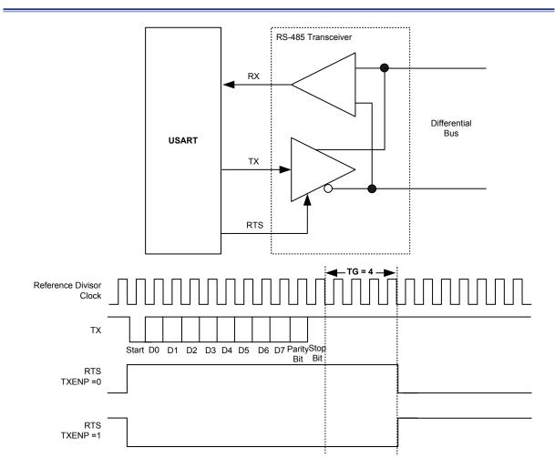
Figure 114. RS485 Interface and Waveform
