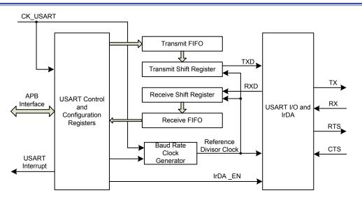
Figure 106. USART Block Diagram
