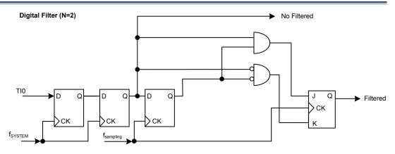
Figure 46. TI0 Digital Filter Diagram with N = 2
