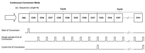
Figure 27. Continuous Conversion Mode
