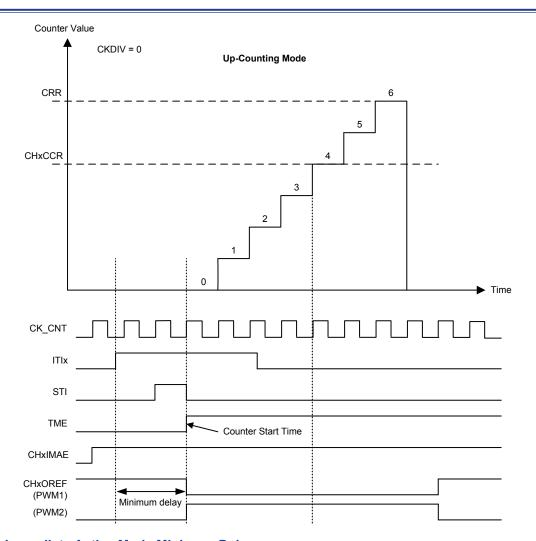
Figure 57. Immediate Active Mode Minimum Delay
