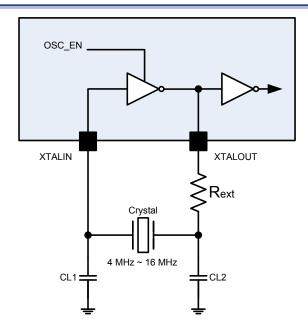
Figure 14. External Crystal, Ceramic, and Resonators for HSE
