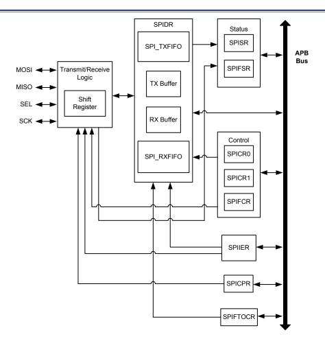
Figure 96. SPI Block Diagram
