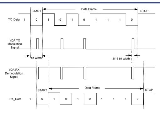
Figure 112. IrDA Modulation and Demodulation
