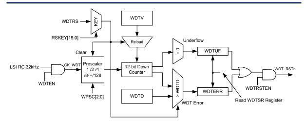
Figure 80. Watchdog Timer Block Diagram
