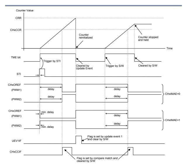
Figure 56. Single Pulse Mode
