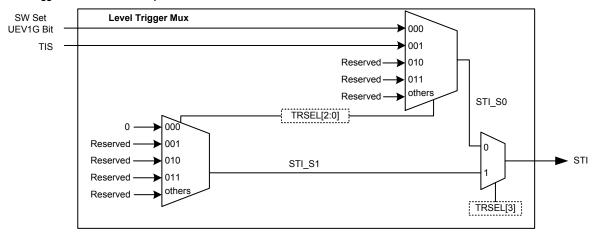
Figure 66. Trigger Control Block
