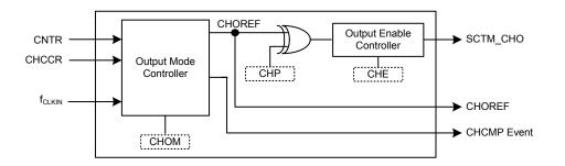
Figure 75. Output Stage Block Diagram
