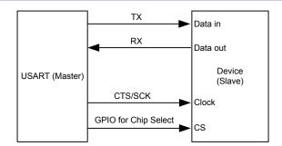
Figure 115. USART Synchronous Transmission Example
