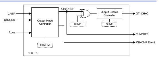
Figure 49. Output Stage Block Diagram
