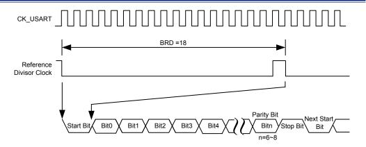
Figure 108. USART Clock CK\_USART and Data Frame Timing
