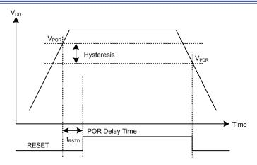
Figure 12. Power On Reset / Power Down Reset Waveform
