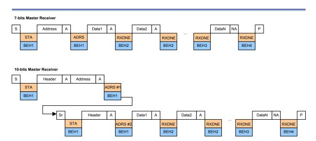
BEH1 : cleared by reading I2CSR register BEH2 : cleared by reading I2CDR register
