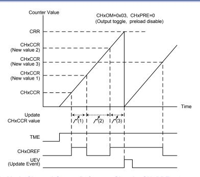
Figure 50. Toggle Mode Channel Output Reference Signal – CHxPRE = 0
