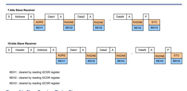
Figure 94. Slave Receiver Timing Diagram
