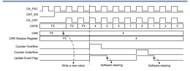
Figure 32. Center-aligned Counting Example
