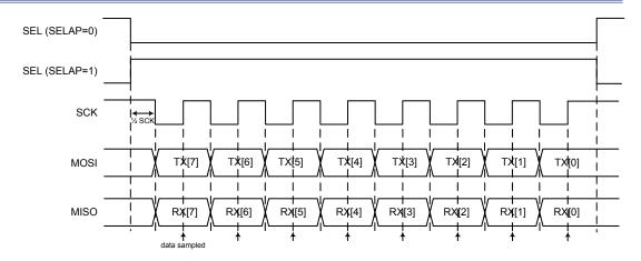
Figure 103. SPI Single Byte Transfer Timing Diagram - CPOL = 1, CPHA = 1
