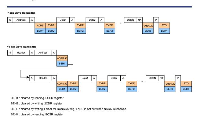
Figure 93. Slave Transmitter Timing Diagram
