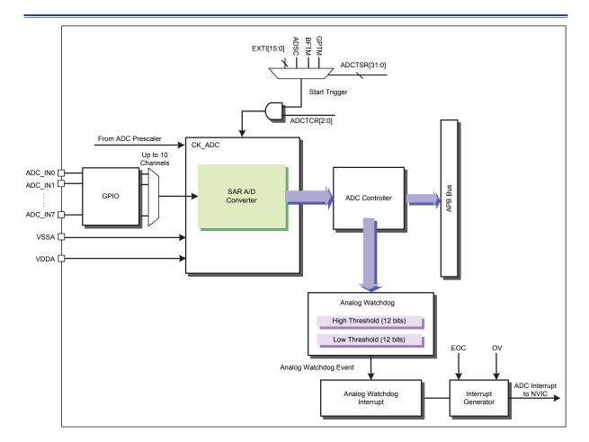
Figure 25. ADC Block Diagram
