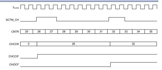
Figure 72. Input Capture Mode
