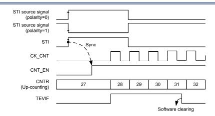
Figure 38. GPTM in Trigger Mode
