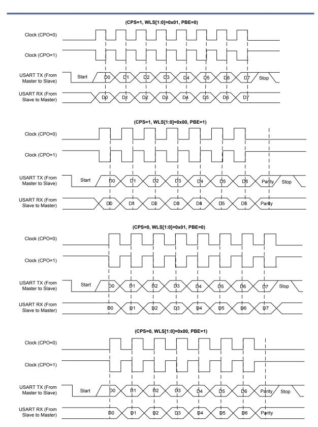
Figure 116. 8-bit Format USART Synchronous Waveform
