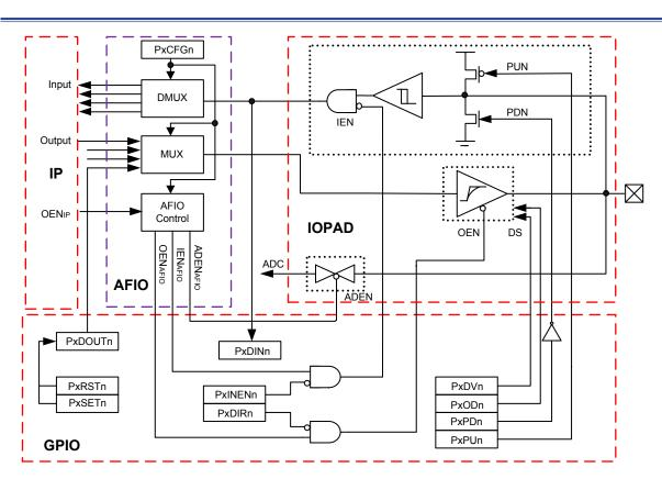
Figure 19. AFIO/GPIO Control Signal
