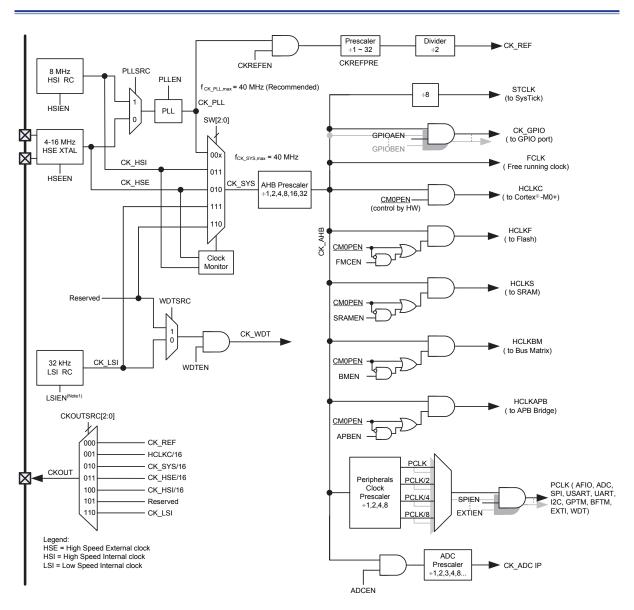
Figure 13. CKCU Block Diagram
