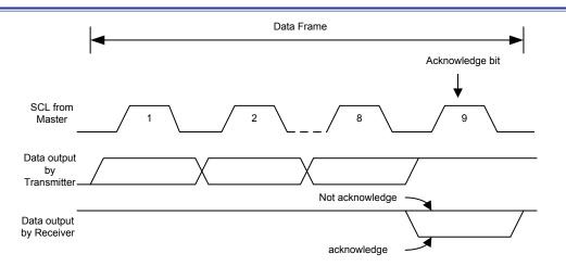
Figure 88. I<sup>2</sup>C Bus Acknowledge
