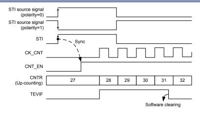
Figure 70. SCTM in Trigger Mode
