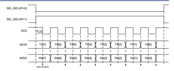
Figure 101. SPI Single Byte Transfer Timing Diagram – CPOL = 1, CPHA = 0
