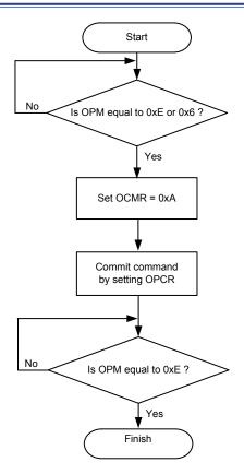
Figure 9. Mass Erase Operation Flowchart
