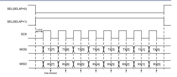
Figure 99. SPI Single Byte Transfer Timing Diagram - CPOL = 0, CPHA = 1
