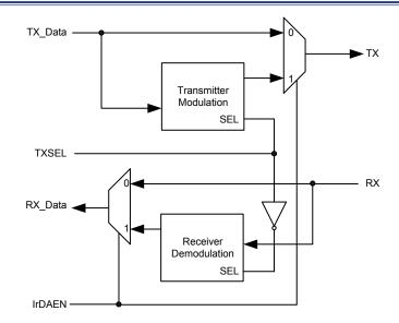
Figure 113. USART I/O and IrDA Block Diagram
