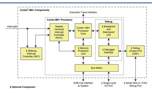
Figure 2. Cortex®-M0+ Block Diagram
