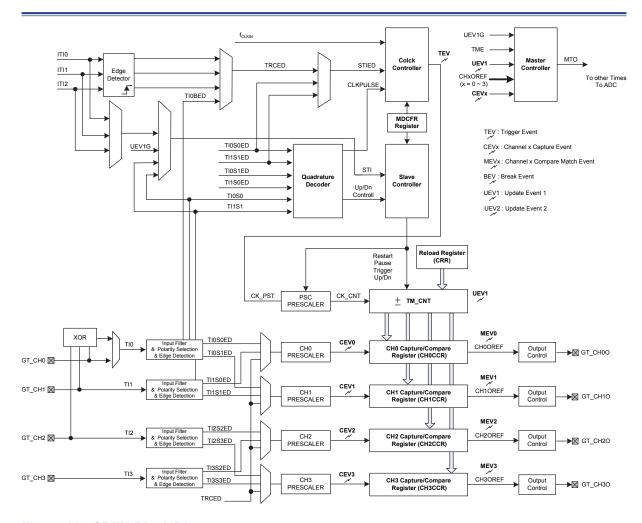
Figure 29. GPTM Block Diagram
