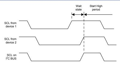
Figure 89. Clock Synchronization during Arbitration
