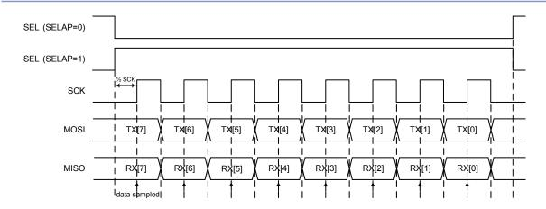
Figure 97. SPI Single Byte Transfer Timing Diagram - CPOL = 0, CPHA = 0
