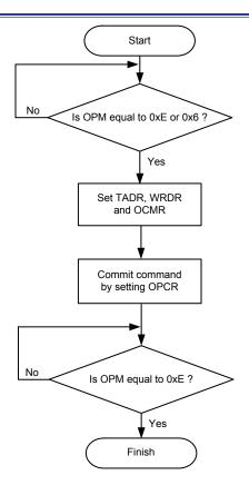
Figure 10. Word Programming Operation Flowchart
