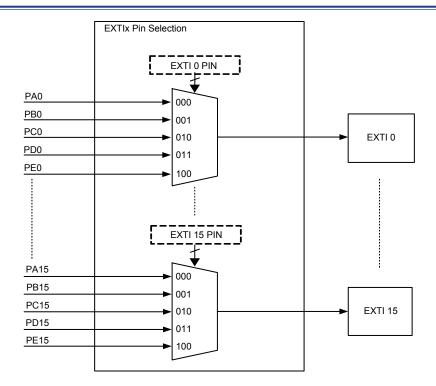
Figure 21. EXTI Channel Input Selection
