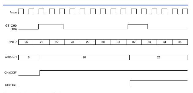
Figure 42. Input Capture Mode
