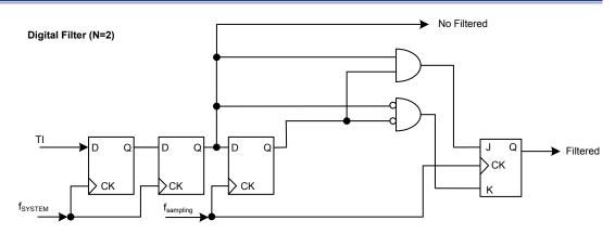
Figure 74. TI Digital Filter Diagram with N = 2
