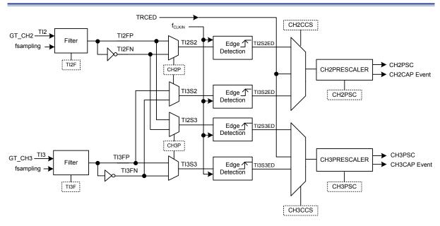
Figure 45. Channel 2 and Channel 3 Input Stages
