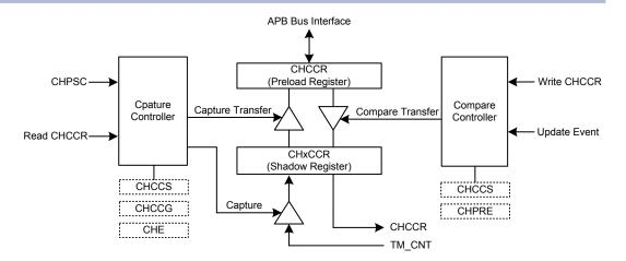
Figure 71. Capture/Compare Block Diagram
