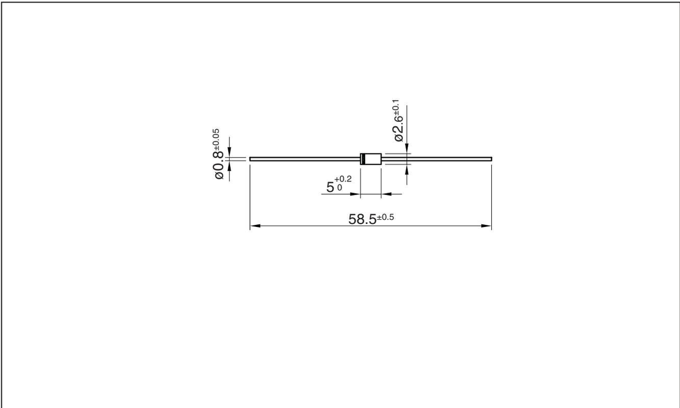
**1.0 Amp. Glass Passivated Junction Rectifier**
