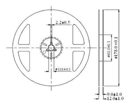
Unit: mm Tolerance:  $\pm 0.25$ mm
