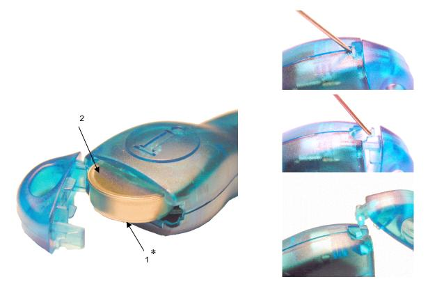
\*Note: The data contact faces down and away from the embossed 'i'. Once the <u>i</u>Button is inserted in the enclosure, snap the end cap over it. The end cap is removed by depressing the release tab with a paper clip, swinging it fully open, and sliding out the hinge.
