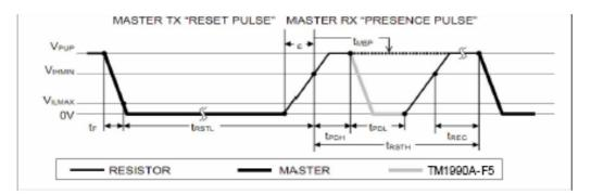
After the bus master has released the line it goes into receive mode (RX). Now the 1-Wire bus is pulled to Vpup via the pullup resistor or, in case of driver by active circuitry. When the V<sub>IHMIN</sub> is crossed, the TM1990A-F5 waits for  $t_{PDH}$  and then transmits a Presence Pulse by pulling the line low for  $t_{PDL}$ . To detect a presence pulse, the master must test the logical state of the 1-Wire line at t<sub>MSP</sub>
