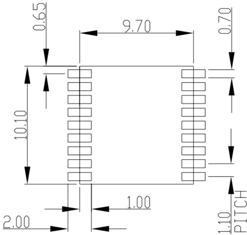
Figure 4: Recommended PCB decal (top view) (Unit: mm)
