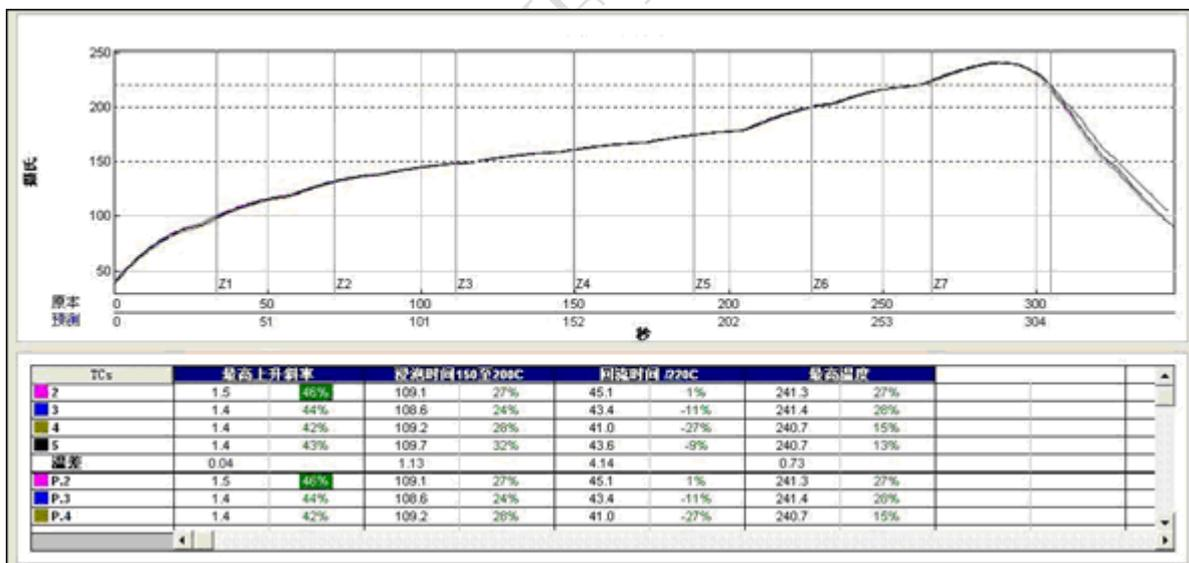
Figure 11: The Ramp-Soak-Spike reflow profile of SIM28M
