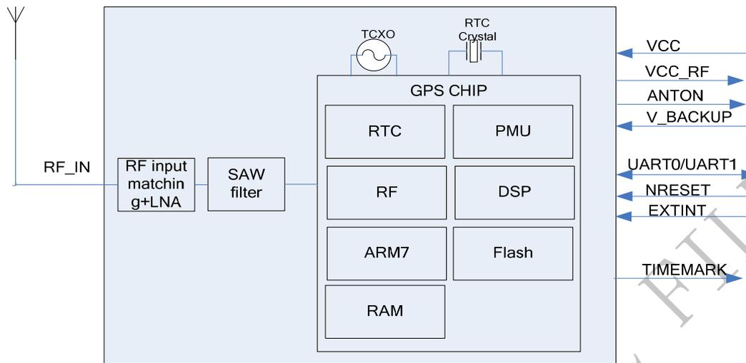
Figure 1: SIM28M functional diagram
