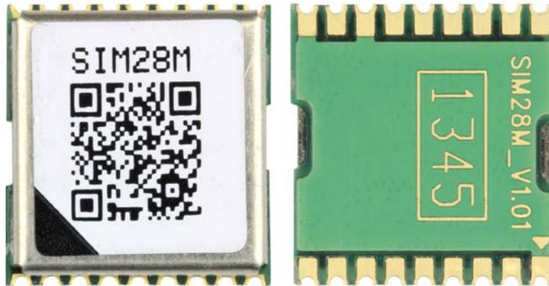
Figure 10: Top and bottom view of SIM28M
