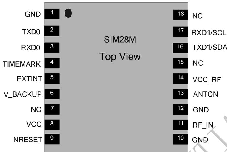
Figure 2: SIM28M pin out diagram (Top view)
