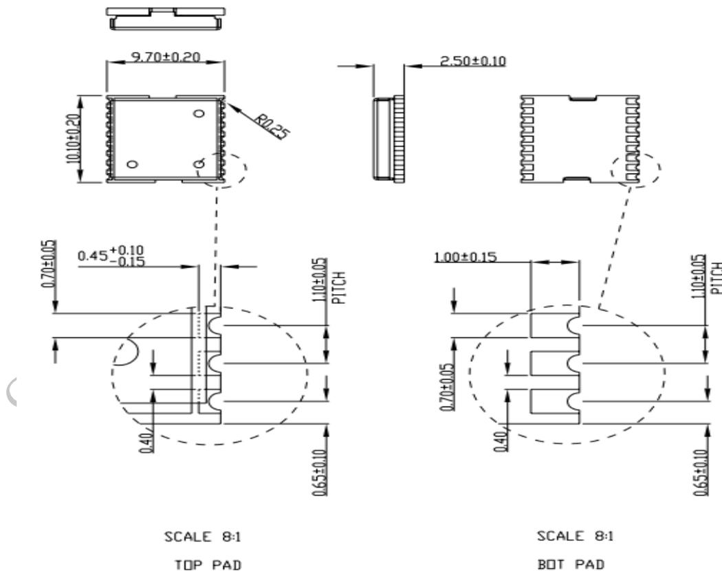
Figure 3: SIM28M mechanical dimensions (Unit: mm)
