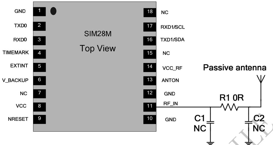
**Figure 6: SIM28M passive antenna design**
