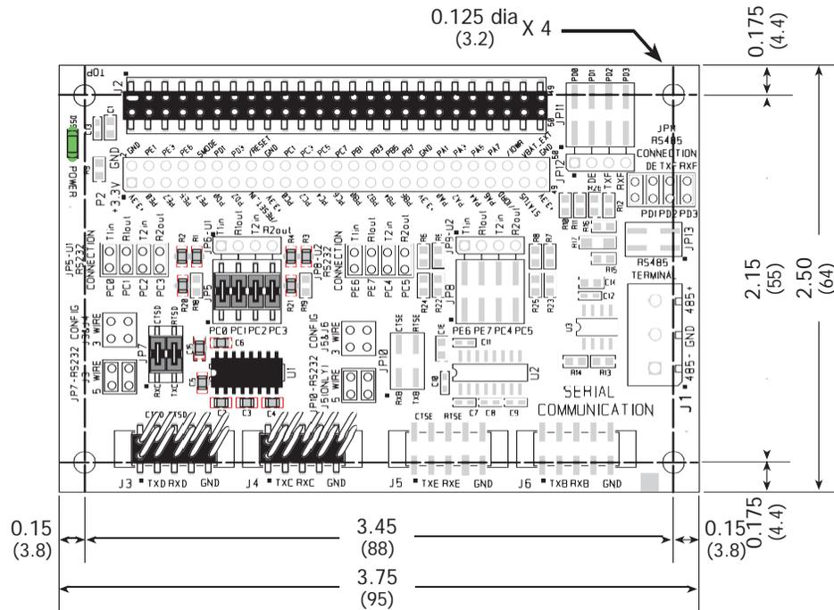
**Figure E-2. Serial Communication Accessory Board Dimensions**
