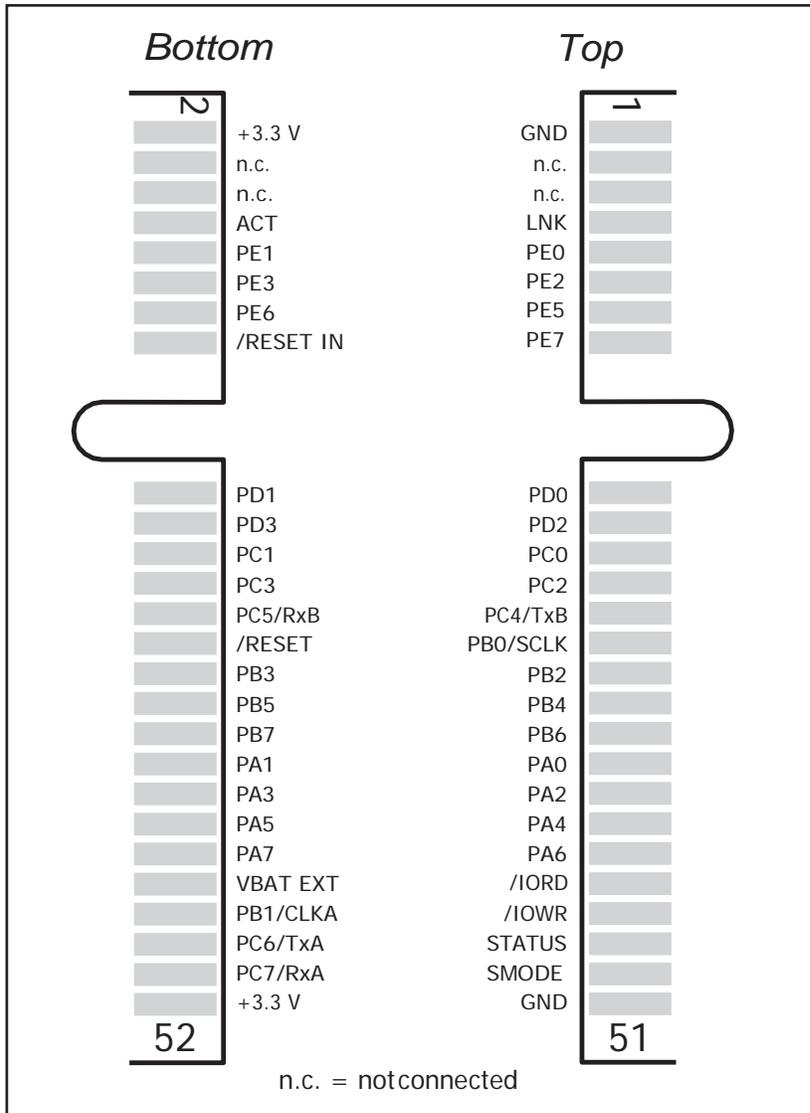
Figure 9. RCM5600W Pinouts
