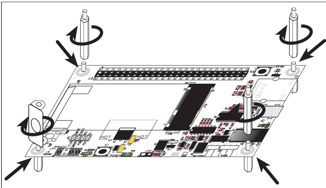
**Figure 2. Insert Standoffs/Connectors**
