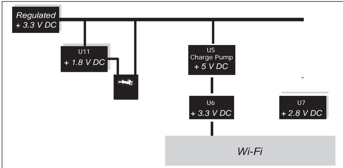
Figure F-2. RCM5600W/ RCM6600W Onboard Power Supplies
