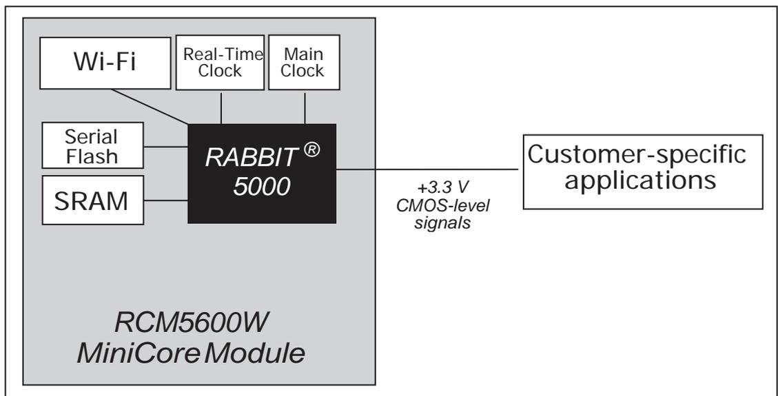
**Figure 7. RCM5600W Subsystems**
