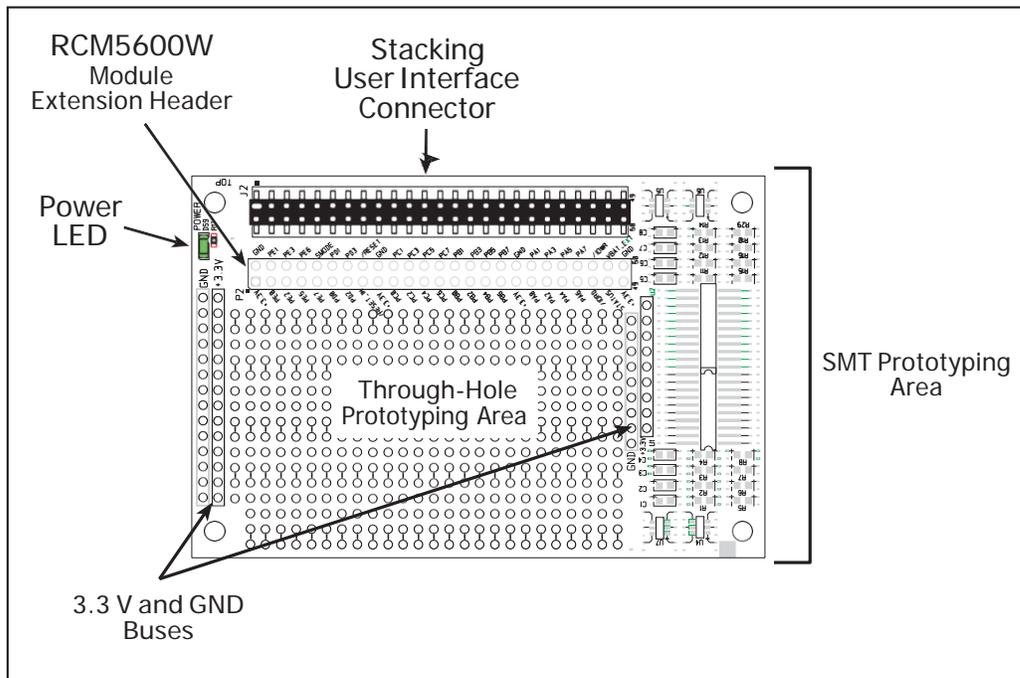
*Figure C-1. Prototyping Board*
