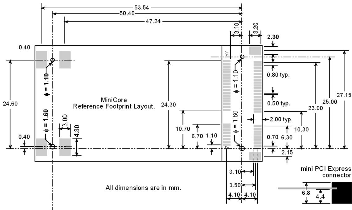
**Figure A-4. PCB SMT Footprint for Pinrex and FOXCONN Connectors**
