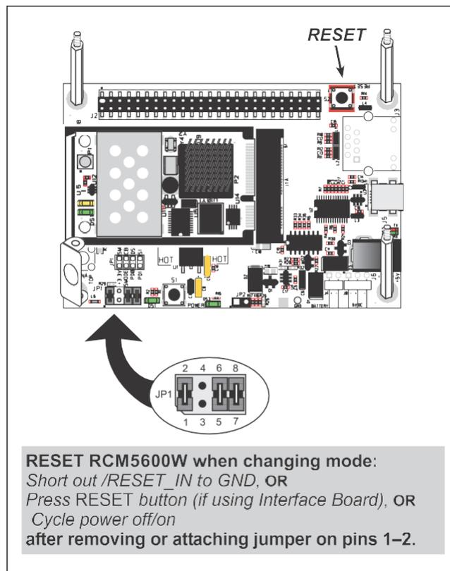
Figure 14. Switching Between Program Mode and Run Mode
