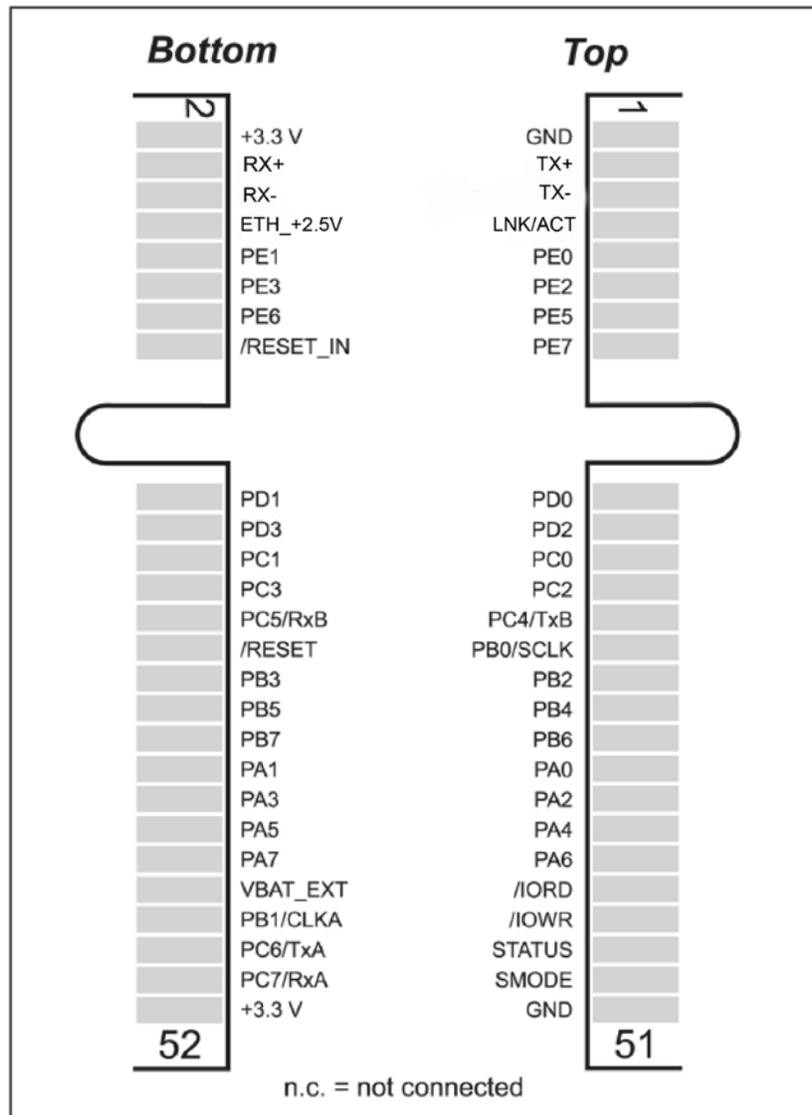
**Figure 10. RCM6600W Pinouts**
