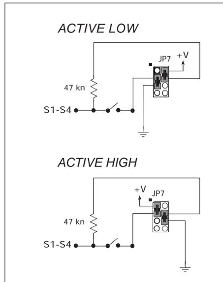
**Figure D-5. Pushbutton Switch Configuration**
